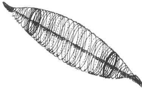
Figure 28. First Forward Mode with Load On Pad Bearing.
